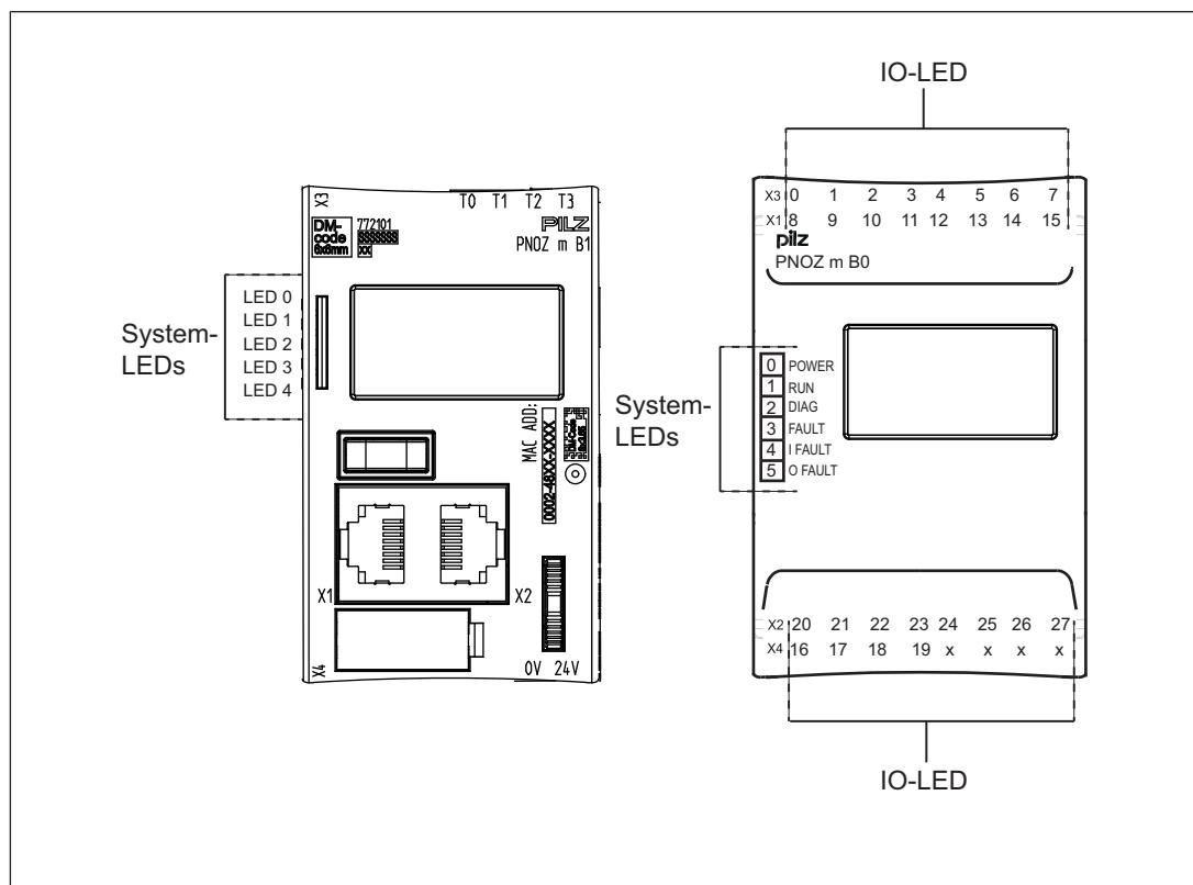
Assignment of the I/O LEDs and system LEDs to the LEDs on the right-hand expansion modules:
