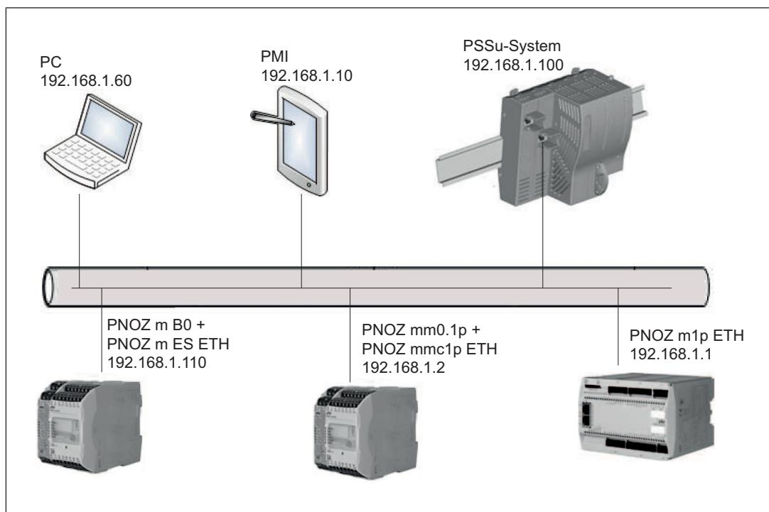
The configurations required for Modbus/TCP are fully pre-configured in the PNOZmulti 2 operating system. All that's necessary in the PNOZmulti Configurator is to activate the virtual inputs and outputs (see PNOZmulti Configurator's online help, under "Display and edit module selection").
