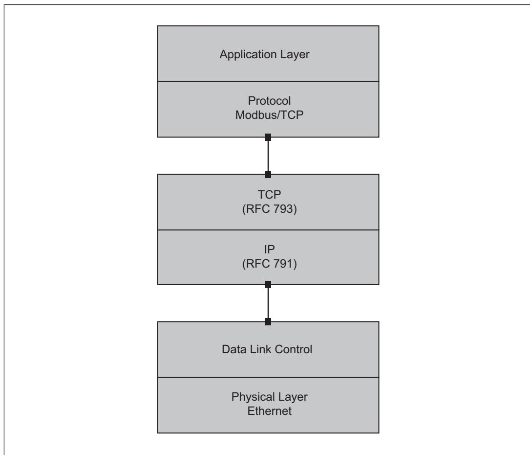
Modbus/TCP is a protocol based on Industrial Ethernet (TCP/IP over Ethernet). It is one of the protocols with Client/Server communication. Data is transferred via a request/response mechanism using function codes (FC).
